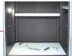
TUBOSCAN S 60 for fast and precise measuring of small pipe bending parts.
