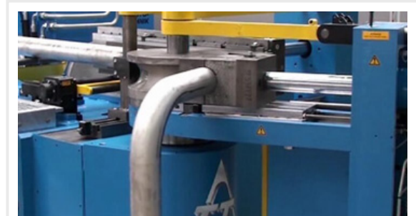
Fully automatic and precise bending of pipes up to Ø 140 mm.
