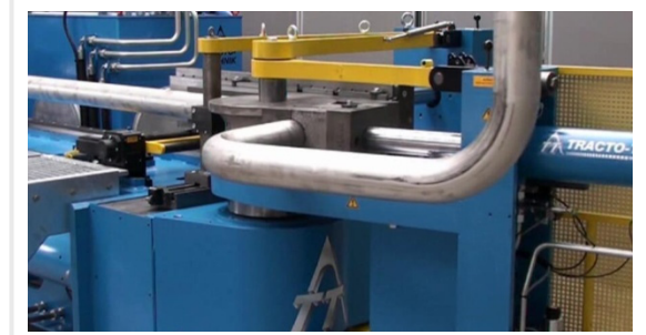
Application example: stainless steel pipe Ø 114.3 x 3.5 mm
