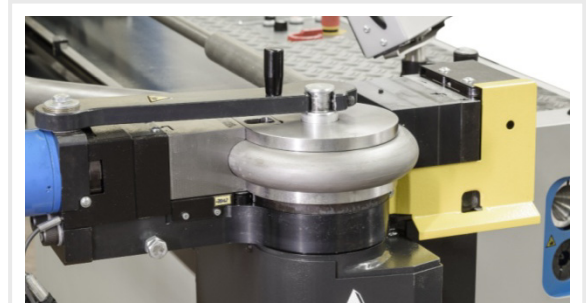
The TUBOMAT's bending head with the optimized tooling concept.
