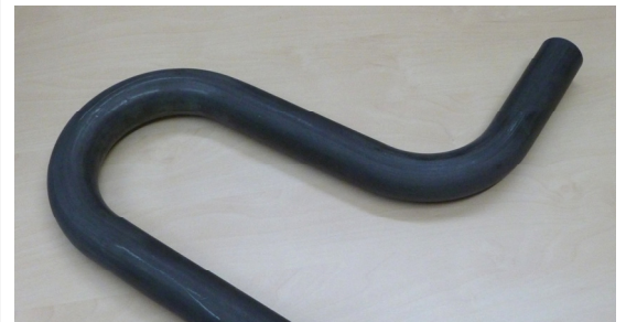
Application example: steel pipe \varnothing 42.0 x 3.0 mm
