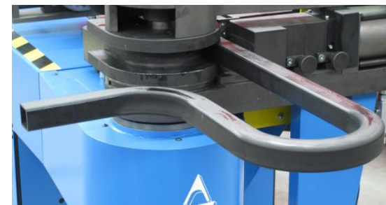
Application example: square pipe, mild steel □ 40.0 x 40.0 x 3.0 mm
