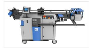
Up to five pipe processing functions can be integrated: Bending, sawing, deburring, cutting-ring assembly, flaring.
