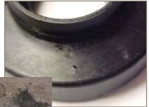
Pitting on filter end-cap
