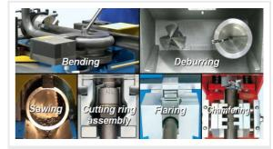
Up to six working functions for safe hydraulic piping integrated in one compact and mobile machine.
