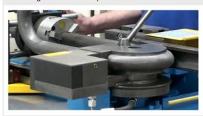
Application example: hydraulic pipe, mild steel Ø 42.0 x 3.0 mm
